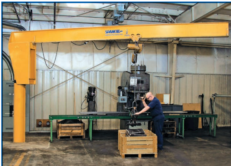
A worker lifts parts into a metalworking machine using a Spanco ½-Ton 101-Series Freestanding Jib Crane.
