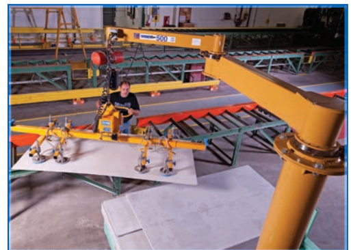
A Spanco 500-Pound Freestanding Articulating Jib Crane with an inverted outer arm and vacuum attachment for easy lifting
