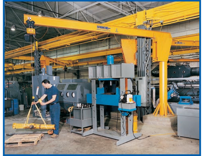
A One-Ton Spanco Freestanding Jib Crane used for shipping and assembly.
