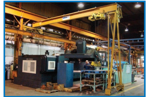
A Spanco 3-Ton Single Leg Gantry Crane with one end supported overhead and one end traveling along the floor.
