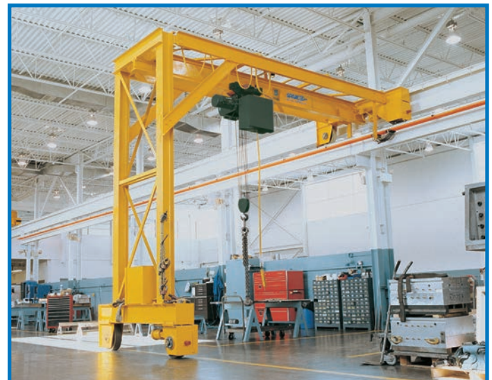
A Spanco Motorized 5-ton Wide-Flange Single-Leg Gantry Crane with an overall span of 20 feet and 15 feet under the beam.
