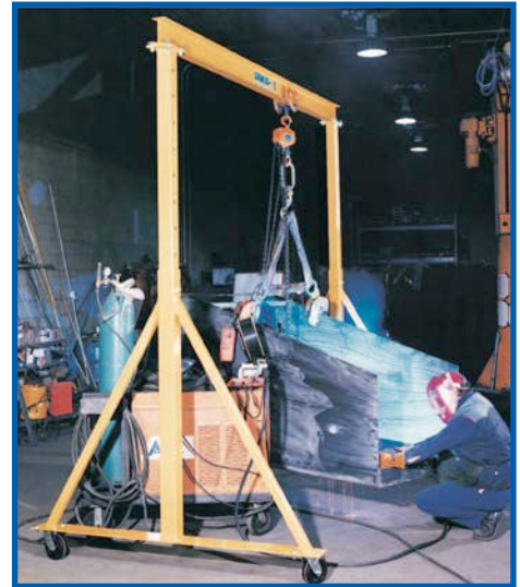
Spanco E-Series Gantry Cranes are popular among welders and other fabricators needing simple stable highly mobile lifting solutions
