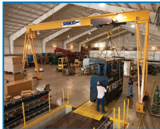
A Spanco 10-Ton PF-Series Gantry Crane with power drive using guide angle for easy travel over a fixed route.
