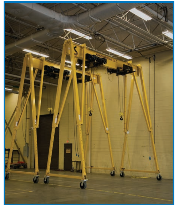
Dual Spanco T-Series Gantry Cranes
