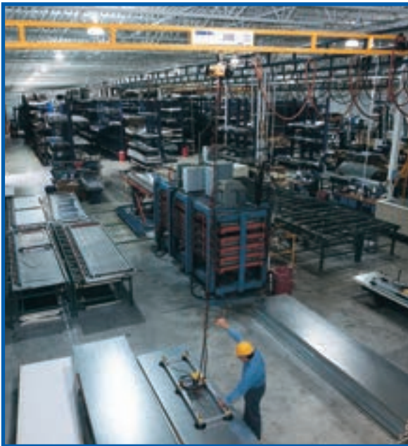
A refrigerator manufacturer using a 250-pound capacity Spanco Ceiling-Mounted Bridge Crane.
