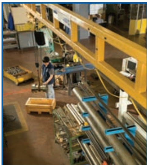
A coupling manufacturer installed several 4,000-pound capacity Spanco Freestanding Bridge Cranes to allow workers to move heavy loads from one work area to another with precision and accuracy.
