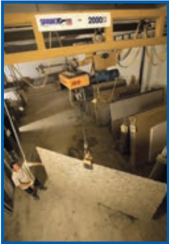
Storage and retrieval of granite countertops is a one-man task using this 2,000-pound capacity Spanco Freestanding Bridge Crane.
