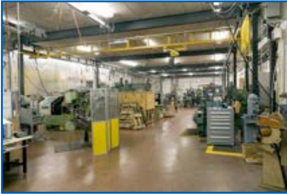
An example of the enormous coverage area possible with Spanco Bridge Cranes. In this case, one freestanding system provides overhead lifting for virtually every workstation in the shop.
