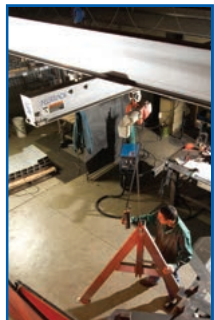
Alu-Track system with aluminum runway and bridge
