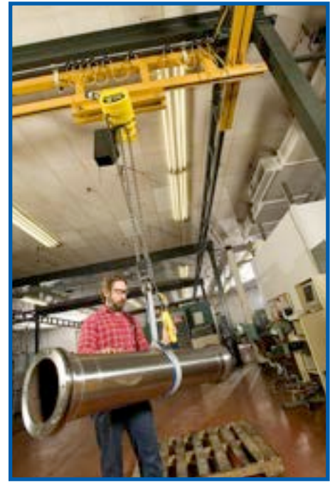
A 4,000-pound capacity Spanco Freestanding Bridge Crane carefully lifts and moves an expensive machined part.
