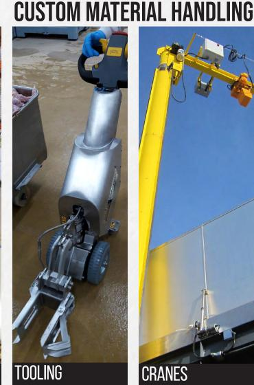
In some cases, the existing equipment within a facility can be fitted with the right tooling to provide a winning solution. This client needed help designing a hitch that worked with a tugger and the industry standard carts in their facility.
