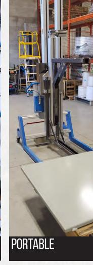
A manufacturing client was in need of a portable solution for moving heavy metal sheets from one area to the other without the use of a crane. We were able to design an attachment that worked with an existing standard product (Lift-O-Flex) as a solution.
