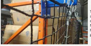
The flue space between racking systems is often an area that sees a high volume of product falls and damages that workers are unable to access. Our Rack Netting System can be installed within this space to help reduce product loss and keep products from getting mixed up with another pallet load.
