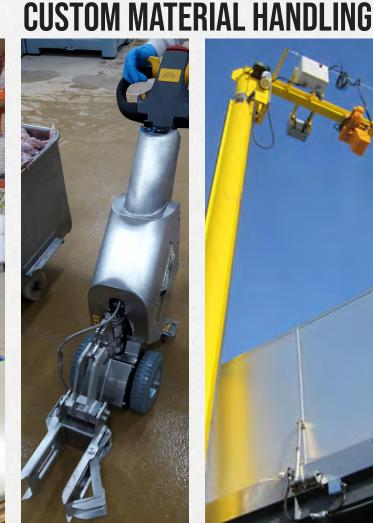
In some cases, the existing equipment within a facility can be fitted with the right tooling to provide a winning solution. This client needed help designing a hitch that worked with a tugger and the industry standard carts in their facility.
