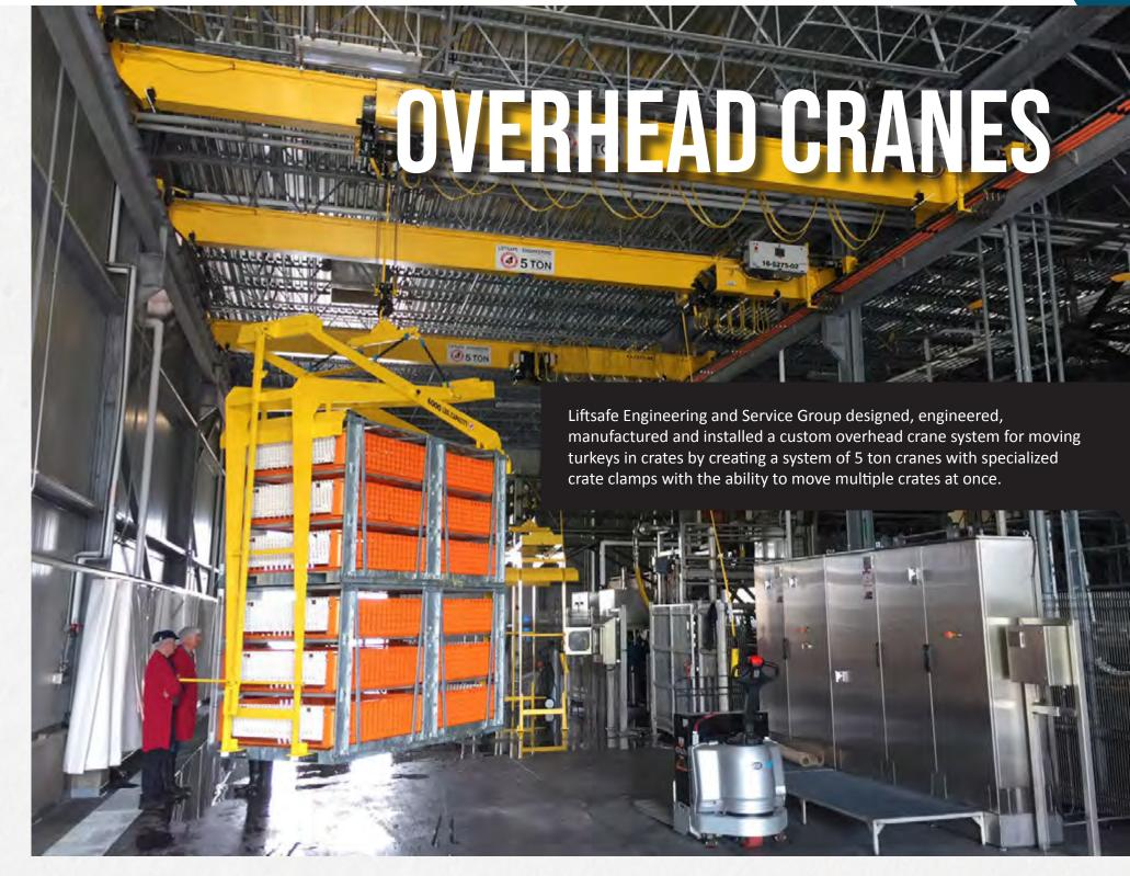
Liftsafe Engineering offers a wide variety of overhead crane systems. These lifting systems are manufactured with elevated parallel runways, which typically run the full length of the facility. A hoist is then used to lift and handle the load as it travels along the span of the bridge. Our systems offer lifting support for loads ranging anywhere from 1 to 100 tons (depending on span), with custom options available in both top running and under running cranes.
